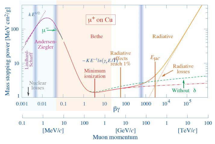
Muon momentum range is typically  $100 \sim 300 \text{ MeV/c}$  for ionization cooling (HF solenoid final channel uses p  $\sim 50 \text{ MeV/c}$ )
