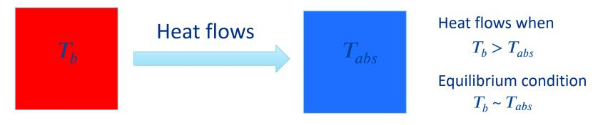
$$\frac{dQ}{dt} = \dot{Q} = h \cdot A \cdot \left( T_b - T_{abs} \right)$$
