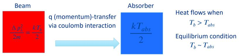
How to effectively generate high transverse momentum in a beam?
